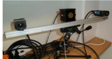
(a) A TOF-stereo setup
