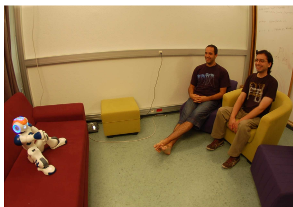
Fig. 1: A typical scenario in which a companion humanoid robot (NAO) performs audio-visual fusion in an attempt to detect the auditory status of each one of the speakers in the room. The system described in this paper processes the raw data gathered with the robot's camera and microphone pairs. The system output is a speaking probability of each one of the actors together with the 3D location of the actors' faces.
