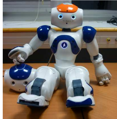
Fig. 6: Within this work we used a new audiovisual head that is composed of a synchronized camera pair and two microphones. This “orange” head replaces the former “blue” head and is fully interfaced by the RSB middleware described in this paper.
