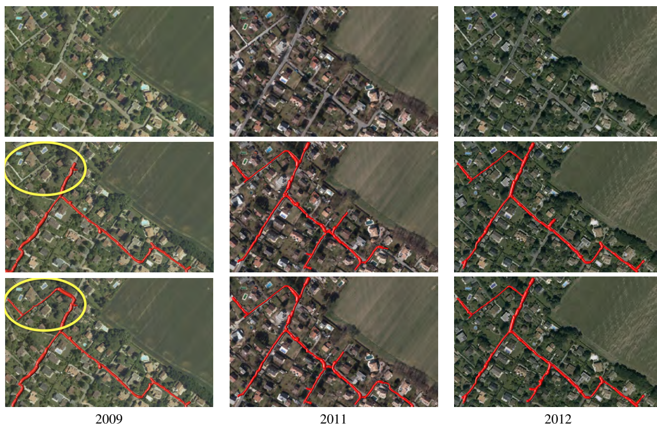
Fig. 4. Road delineation. First row. Images acquired in 2009, 2011, and 2012. Second row. Delineations without temporal consistency. Third row. Delineations with temporal consistency enforced. Note the added road fragments within the overlaid yellow ellipse.
