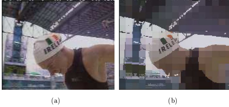
Fig. 2. Robust filtering using the mean shift algorithm: (a) original image (b) filtered image (every neighbourhood pixel replaced by the mode of the density function it converged to)
