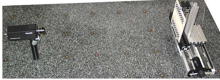
Fig. 4. Experimental setup. The camera and the moving table mounted on granite slab.
