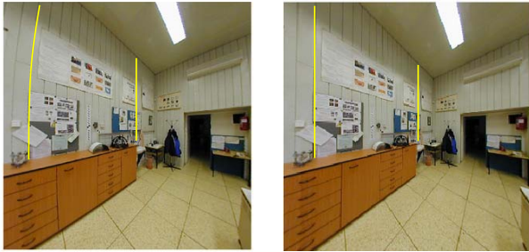
Figure 12: Image with 120^\circ angle of view reprojected to a plane. Left: approach by [6]. Right: our method. Notice that with our method all lines are straight.
