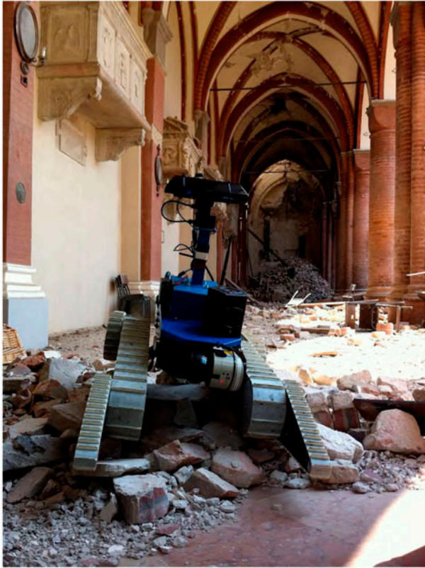
Figure 20. NIFTi UGV with a rotating SICK-Laser (LMS100), a LadyBug3 omnicaam, active flippers and active/passive bogeys, IMU, GPS, and a static mast mounting a PTU with a Kinect sensor.
