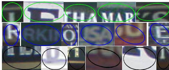
Fig. 1: An example of features whose visual words were learned to predict the position of a text line (from top to bottom): top of the text line, both top and bottom, and bottom.
