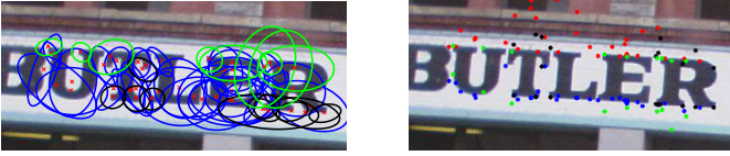
Fig. 3: Three types of visual words are learned (left): predicting only top of the text line (green), predicting only bottom of the text line (black) and predicting both top and bottom (blue). Feature classification based on location. Each feature provides an estimate of the position of the text line (right). Estimates from features estimating only top (green) or bottom (black) are typically reliable.
