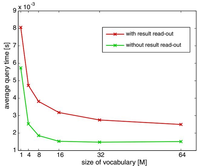
**Fig. 10** The dependence of the query time on the vocabulary size. The times were measured on the Oxford 105k dataset. To measure the speed of inverted file, we are not using spatial verification, alternative words, or query expansion. The green line shows times measured without sorting the documents according the score and copying them to the output.
