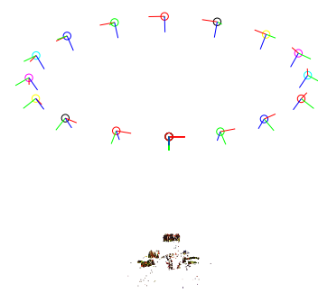
Figure 5. Correct 3D reconstruction of cameras in a “turntable configuration” by our method. This is a degenerate configuration for general 6-pt algorithms which often occurs with causal photographers taking pictures of 3D objects.
