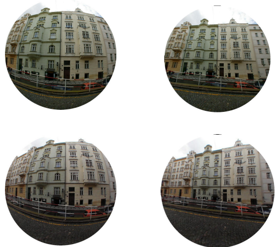
Figure 5. Real data, 60% cutouts from omnidirectional images. (Left) Input images with different radial distortions for camera 1 (Top) and camera 2 (Bottom). (Right) Corrected images.
