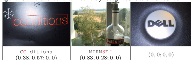
Figure 7. Limitations of the proposed method. Reflection of a flash is too strong so the letter “n” is not detected as an MSER (left). An unsupported text line shape and letters written on glass not detected as MSERs (middle). Multiple letters joint into one region (right)
