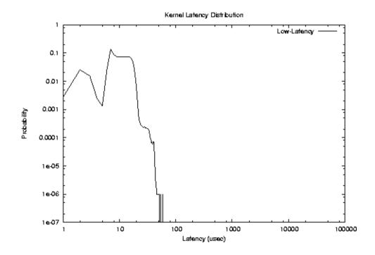
Figure 7-5. PDF of the Latency in the Low-Latency Kernel
