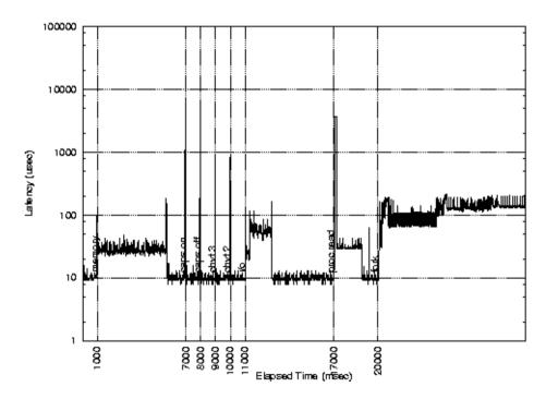
Figure 7-2. Latency in the Low Latency Kernel
