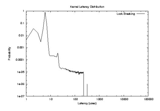
Figure 7-6. PDF of the Latency in the Lock-Breaking Kernel
