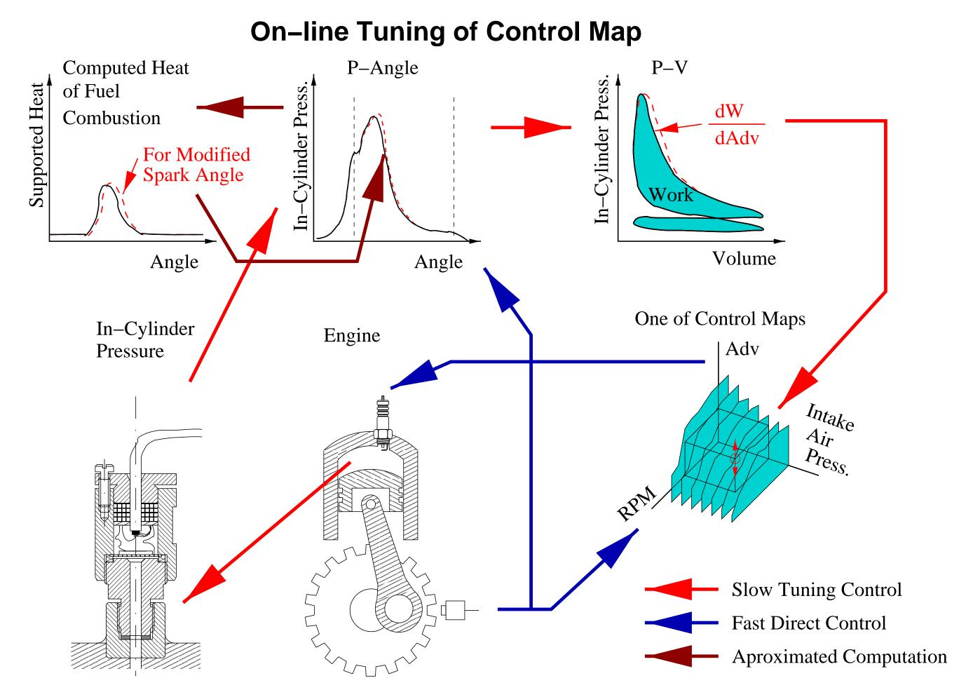
Above described method for optimization of ignition timing for each working state is in preparation for experiments. We have developed additional software for our ECU and designed and produced low cost pressure gauge for experiments.
