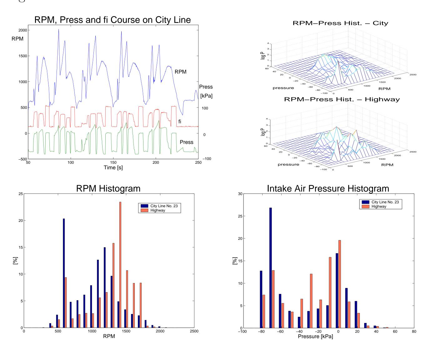
Measured data show the difference between a typical city traffic (acceleration and breaks from one bus stop to other one) and more smooth traffic on an inter-city line on highway. Data measured on Bratislava bus line No. 23 were taken as an example of city traffic.
