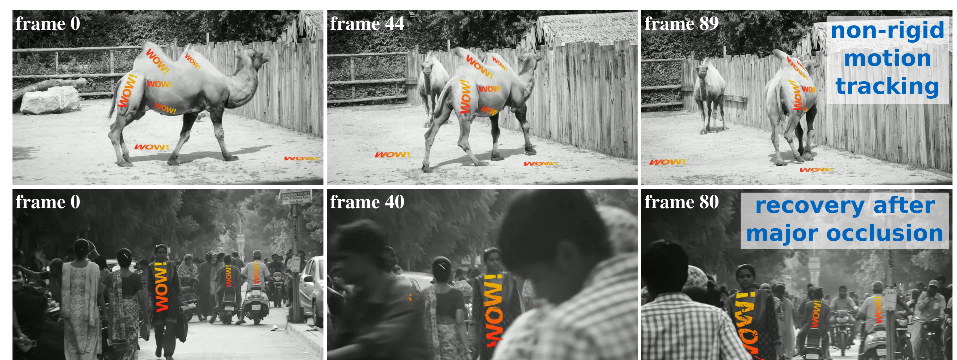
A WOW! logo inserted in frame 0, color propagated by MFT to all frames
