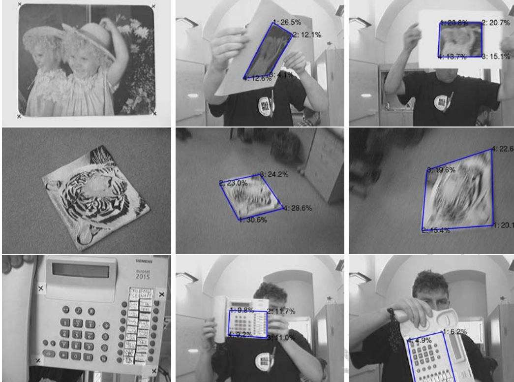
Fig. 6. The left column shows images used for training. The middle and right columns demonstrate some successfully tracked frames with strong motion blur from the testing sequences. Blue rectangle delineates the object. Percentage values in corners are current corner speeds related to the current size of the object upper edge.
