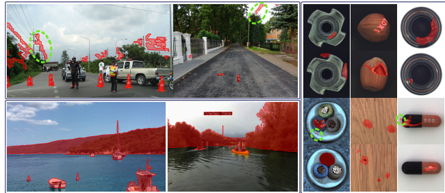
Fig. 1. Examples of PixOOD results for road, maritime and industrial anomaly detection tasks. PixOOD is able to identify anomalous data not even considered, i.e. not labelled, in standard benchmarks, e.g. power cables (not in Cityscapes training classes) or spilled-out content or scratches in insulation.
